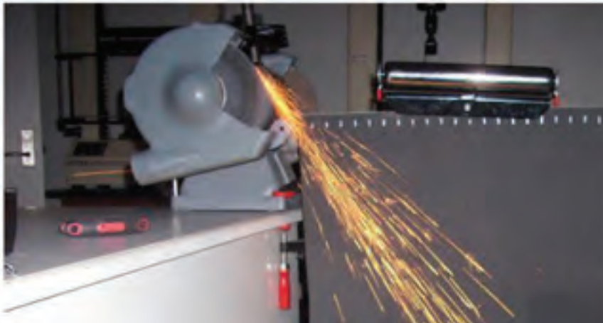
Figure 2: Spark test of a high carbon steel
