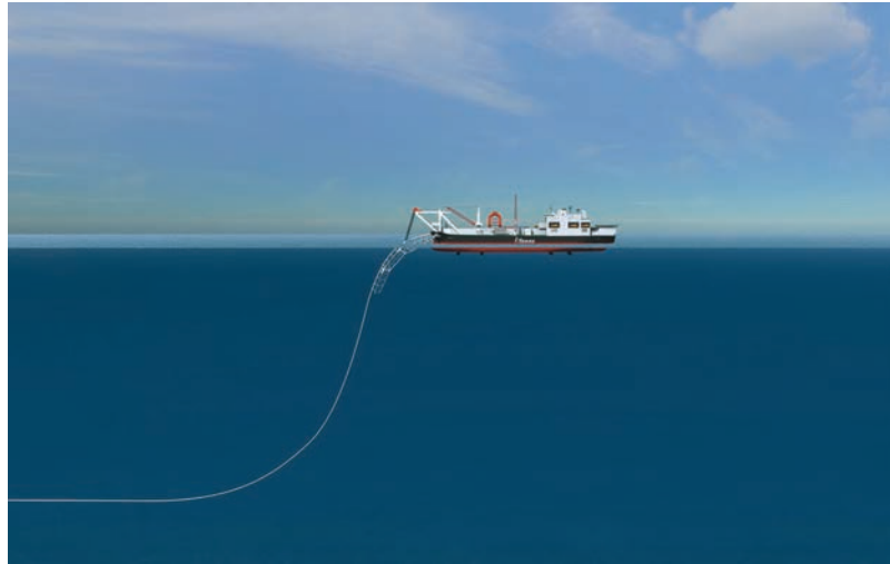
pipe laying vessel
