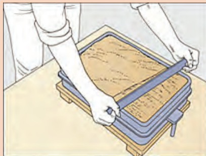
Level the Sand in the Drag .....
