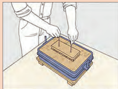
Removing the Pattern .....
