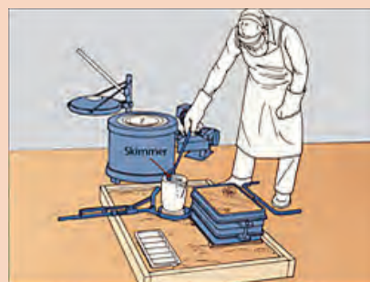
Skimming Slag from Molten Metal .....
