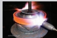
Flame hardening, torch hardening.....
