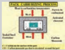
Carburization, cementation, carburizing, carburising.....
