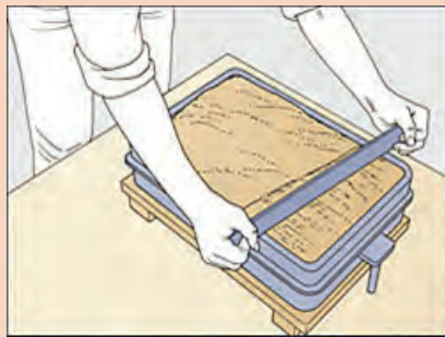
Level the Sand in the Drag .....
