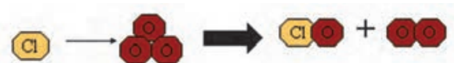
Lone Cl strikes ozone, leaving chlorine monoxide & oxygen molecule, which results in a loss of ozone
