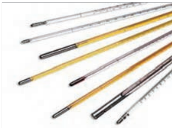
Fig. 26: Laboratory liquid - expansion thermometer
