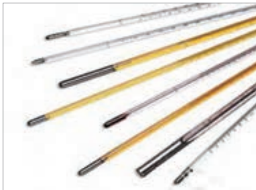
Fig. 26: Laboratory liquid - expansion thermometer
