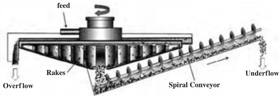
Figure 13.3: Sketch of a Bowl Classifier With Spiral Conveyor For Collecting Sand From The Tank and Discharging to The Launder at The Top End Of The Vessel
